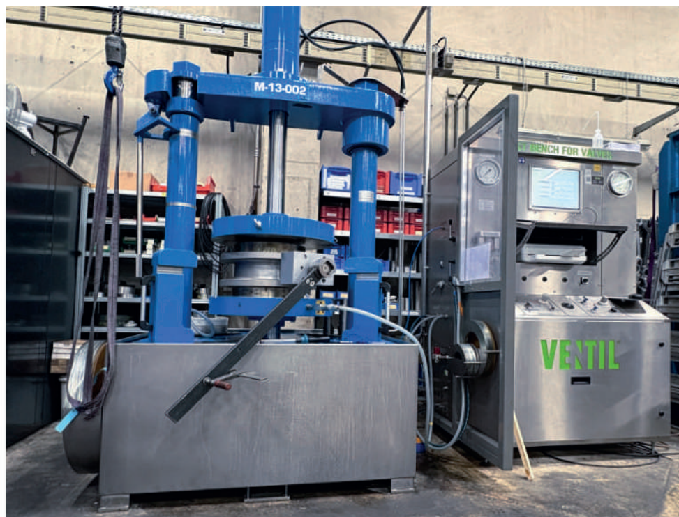
Test bench for air testing: DN 25–DN 600 and liquid testing system up to 400 bar
